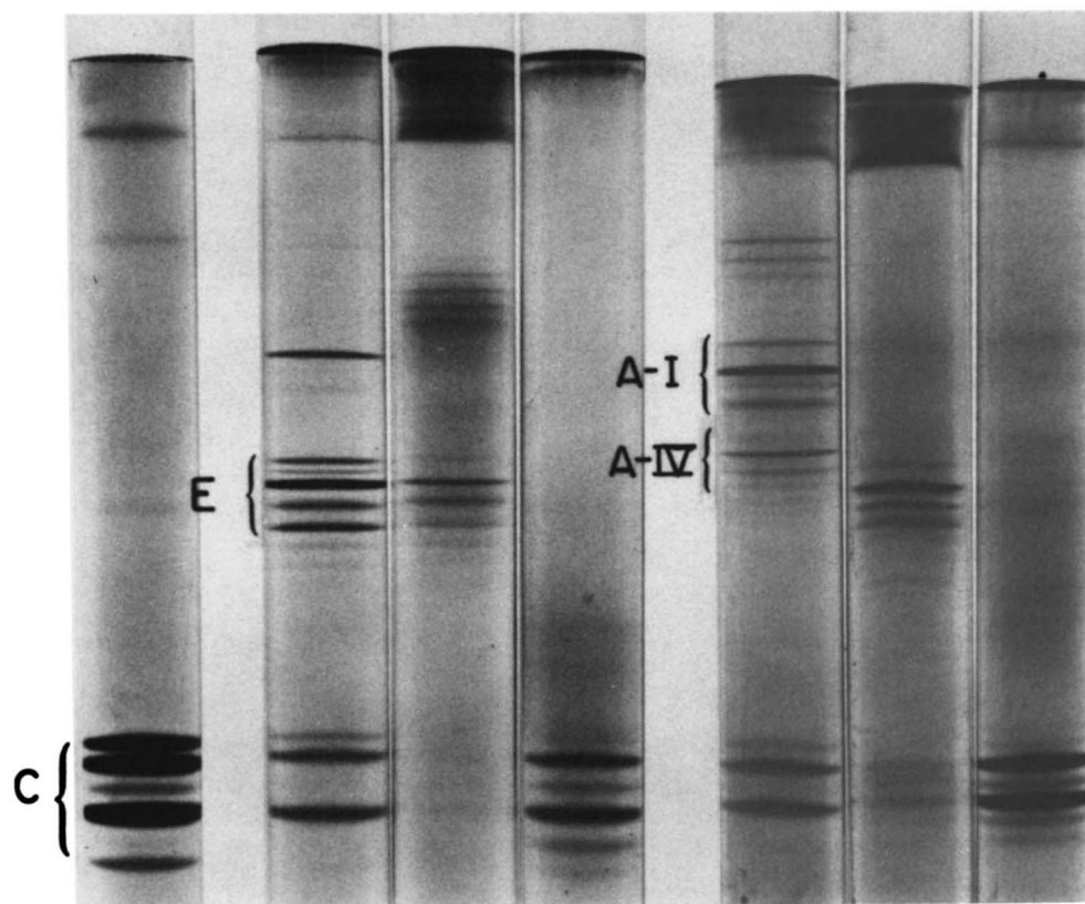
Fig. 7. Isoelectric focusing polyacrylamide gel electrophoretograms of apoproteins. Left, isolated rat C apoproteins. Middle group (from left), rat VLDL, VLDL remnants, and these remnants incubated with C apoproteins. Right group (from left), lymph small chylomicrons, small chylomicron remnants, and these remnants incubated with C apoproteins. In each group apoproteins derived from lipoproteins containing the same amount of [ ^3\text{H} ]CE were applied to the gels. Note that the uppermost of the C apoproteins (C-II) is almost lacking in the remnants incubated with C apoproteins and that virtually no apoE remains.
